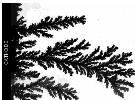
Figure 1. Electrodeposition of copper on a substrate (reprinted with permission from V. Fleury). The quasi-two-dimensional cell is composed of two copper electrodes and a CuSO_4 solution for the electrolyte (sample size 3 \times 2 \text{ mm}^2 ). Only a small part of the sample is shown.
